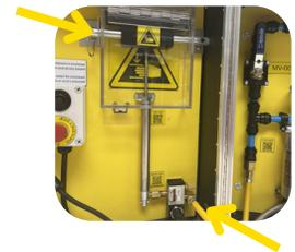
Then insert the rod and insert a padlock into the hole to secure the power source.
